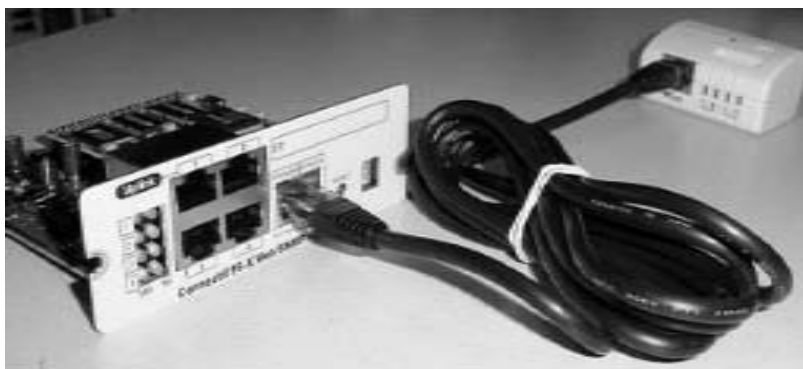
Figure 25. ConnectUPS-X Web/SNMP Module and Environmental Monitoring Probe.
